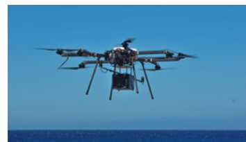
LiteWave Technologies EDGE topobathy LiDAR mounted on the Skyfront Perimeter 8 drone platform.
